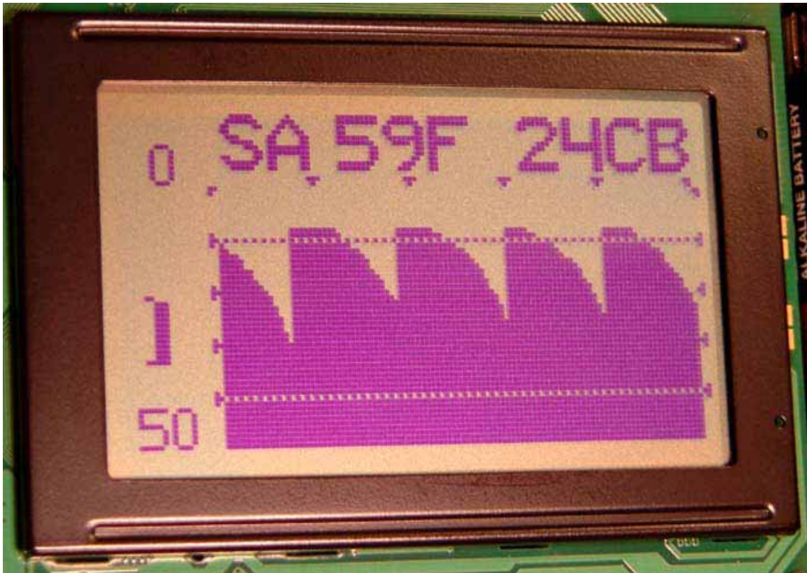
The new AM400 Version 3E average display shown with the protective cover removed.
